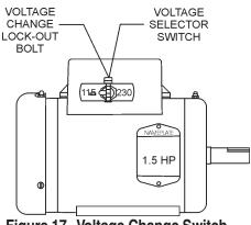
Figure 17. Voltage Change Switch (115 VAC Position)
